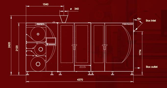
APU (Auto-Packaging-Unit) is an EOL without box erector and lid closer. The machine is prepared to be retrofitted with a box erector and lid closer.
